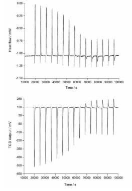
Figure 7 — Typical pulse-FMC data for the ammonia adsorption on Amberlyst 15 at 100 °C and 2ml min–1 flow rate and corresponding TCD data
