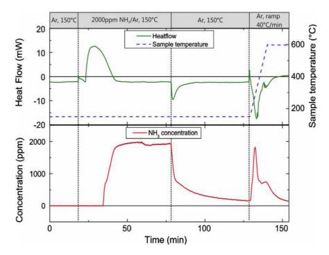
Figure 3 – Thermogram and FTIR signal for an NH3 TPD experiment on a Cu-Beta catalyst
