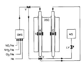
Figure 4 – TC, catalyst; GMS, gas-mixing system; DSC, differential scanning calorimeter; LV, leak valve; MS, mass spectrometer; R, reference; S, sensor; V, valve
