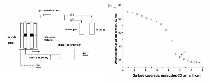
Figure 10 – Schematic representation of the Calvet type DSC with the injection loop and the MS coupling
