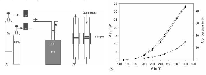
Figure 8-(a) Mixing of the different gases, (b) Gas flow within the quartz tube reactor
