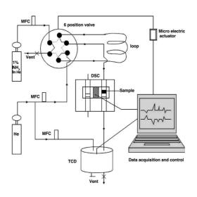
Figure 6 – Pulsed flow adsorption calorimeter system
