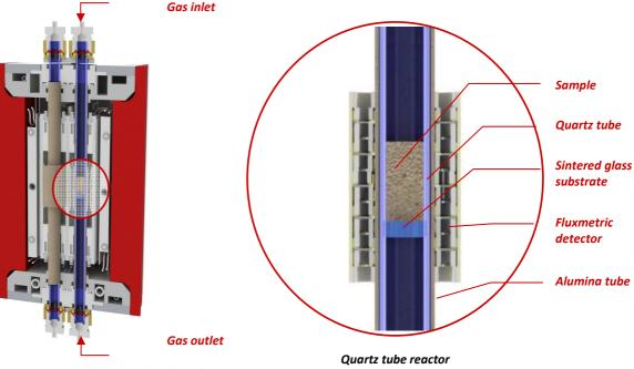
Calvet type DSC cross section in the vertical mode with the quartz tube reactor
