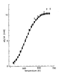
Figure 5 – Heat produced by the reaction of NO, NH<sub>3</sub>, and  $O_2$ , over  $V_2O_5$  on a TiO,  $_2$ /SiO $_2$  catalyst as a function of temperature
